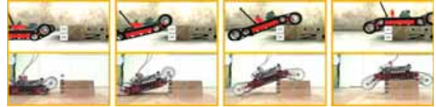
Fig. 8. Simulator evaluation. Top: simulated robot and bottom: real robot.
