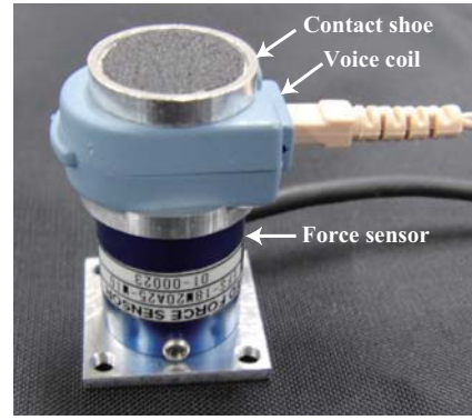
Fig. 7. Pointing-stick interface with a tactile stimulator
