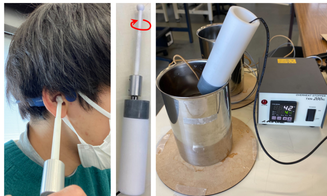
Fig. 1. Experimental apparatus. Left) Experimental scene. Middle) Tactile stimulator for ear. Right) Rod retained in temperature-controlled water.
