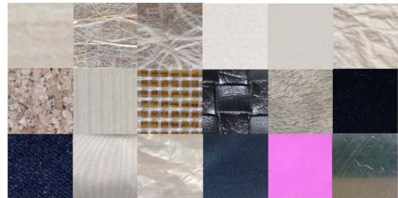
Fig. 2: To measure the force, 18 kinds of material were used. Upper row (from left): wood, coarse Japanese paper, fine Japanese paper, drawing paper, coated paper, and crumpled paper. Middle row: cork, corrugated paper, woven resin wire mesh, fake leather, fake fur, and felt. Bottom row: denim, polyester cloth, polyethylene sheet, rubber, sticky rubber (rubber glove), and flat aluminum
