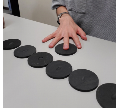
Fig. 1: Experimental scenario; pushing flat and hard plates with a concave or convex at the center.
